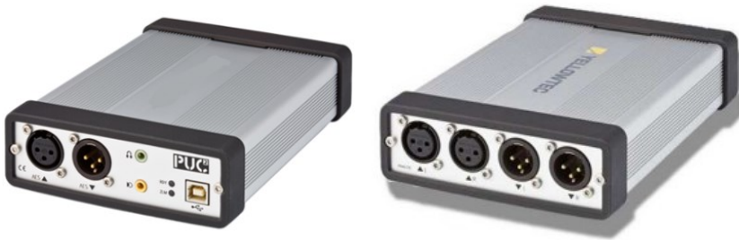
Figure 2-3 CMX-ZG180A external media endpoint (left: front view / right: rear view)
