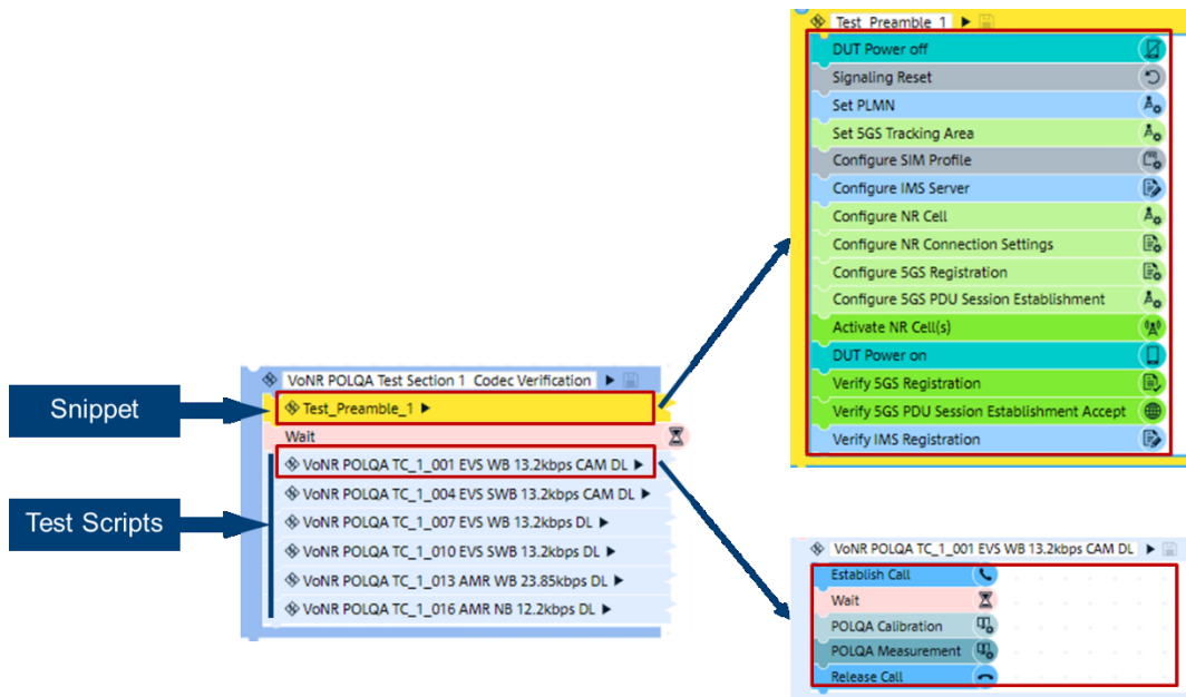
Figure 4-15 Structure of a POLQA test plan in CMsequencer
